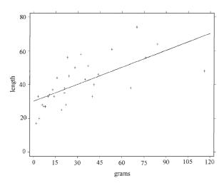
Fig. 1.1.4.b. Correlation of core length and weight. - Korelace délky a hmotnosti jader.
